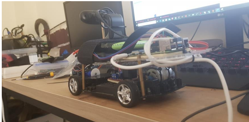
Figure 15. Changing DC motor to a higher torque motor
